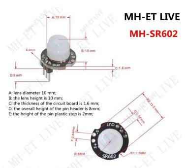
F: photosensitive element pad pitch 2.54mm; G: the pin spacing of the power input and signal output is 2.54mm; R: the board has a radius of 8 mm;
